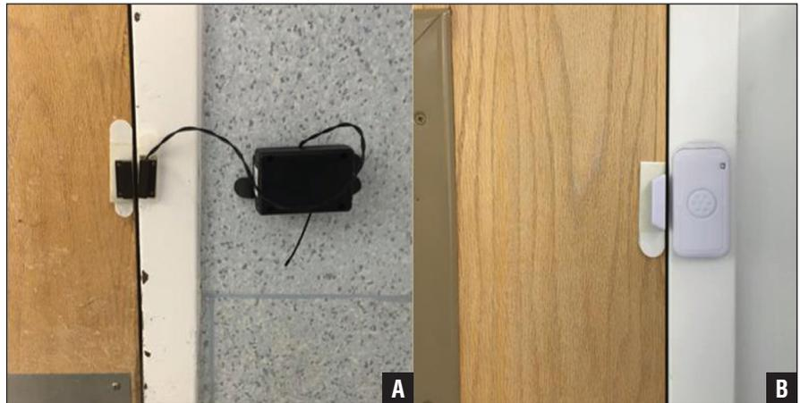
**Figure 2:** A wireless magnetic door counter (Wireless open-closed sensor; Monnit Corporation, Murray, Utah) was placed on the inner substerile door (A). A battery-powered alarm was placed on the inner substerile door (B).
